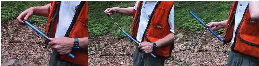
Figure 3. How to assemble an increment borer
